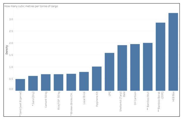
Partners are requested to respect vehicle payload and volumetric capacity. Even if trucks do not reach their maximum payload, they should not be loaded beyond their cargo compartments. Overloading effects vehicle balance and can cause them to roll over.
